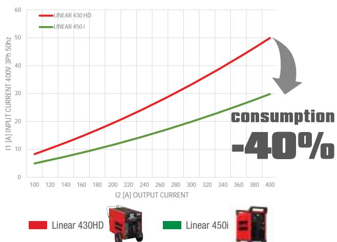
**EN/** Welds more, consumes less! Inverter technology reduces consumption by 40% compared to models with electromechanical technology.
