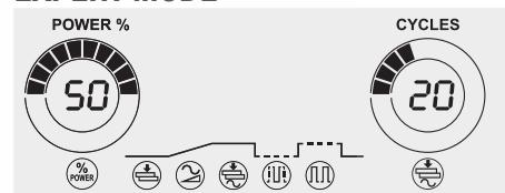
Setting of different spot welding parameters
