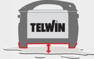
ELEVATED STRUCTURE VS WATER & DUST
